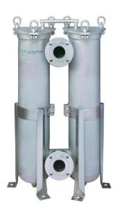
MEY's Duplex Bag Filter Housing is designed with two single bag filter housings fitted together at the inlet and outlet by a butterfly valve or ball valve assembly. Allows for continuous process flow even during filter bag change-outs. Vessels offer the flow and loading capacity of a multi-bag vessel at a more economical cost.
