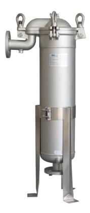
MEY's TOPLINE single bag filter stainless steel housing with the design of top inlet, requires less headroom and directs liquid flow through the cover which improves sealing, reduces product loss and makes filter bag change-outs cleaner. As standard, the MTBH series is provided with heady duty adjustable mounting bracket support legs and SS filter basket supplied to support for the filter bag.
